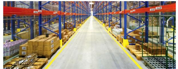
"Sufficient safe clearances" must be provided where mechanical equipment is used. The width required will vary depending upon how the aisle is utilized in the workplace - Aisles that utilize forklift and truck traffic will need to be wider than aisles for pedestrian traffic. **A good average aisle width is 36 inches.**
