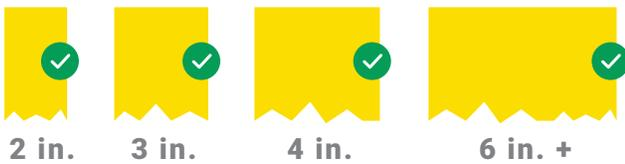
To ensure maximum visibility/awareness, **the required minimum width required for facility aisle and floor marking lines is 2" wide**- therefore, any width above that is considered acceptable by OSHA and ANSI. Most typical applications use tape or painted lines with **2" - 6" widths**.
