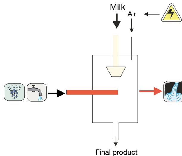
The advantage offered by this system lies in the short period of heating, which implies very moderate treatment of the product. A disadvantage is the need of high-quality steam. The capacity for recovery of thermal energy is only 40-50 per cent.
