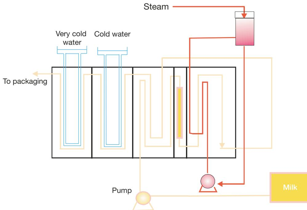
This heating system has the advantage of permitting high recuperation of heat (80-90 per cent). The main inconveniences are the possibility of damaging the product from overheating and the difficulty of cleaning deposits on the exchangers.
