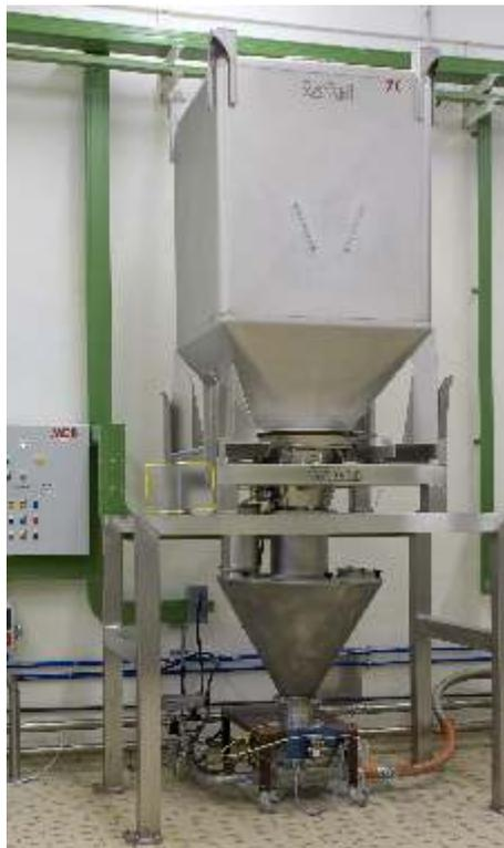
IBC Feed to Pneumatic Conveyor
