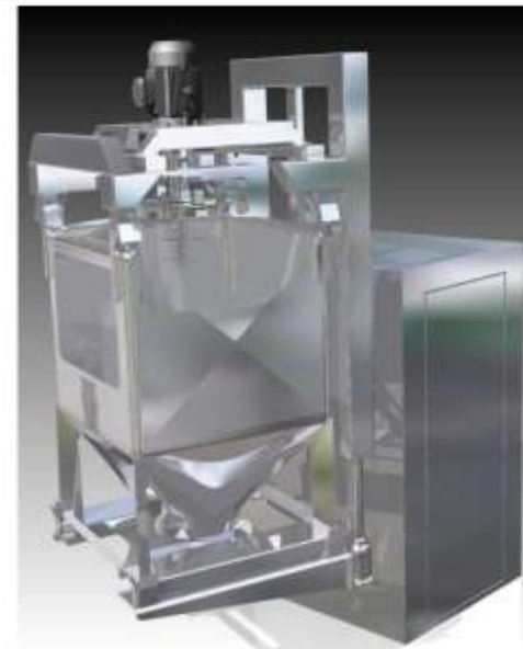
Fig 3: IBC batch mixer with 'high shear' capability.
